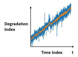
Fig. 6. The trend (orange) of the degradation index in RUL prediction is monotonic. However, the sequence might contain anomalous data, depicted as datapoints with great difference compared to the trend. Anomalous data are removed using multi-pass training to improve performance.
