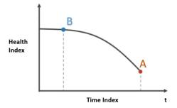
Fig. 1. Health index of an asset over time. Given two measurement points at time index  $t_A$  and  $t_B$ , we can assume the health index at  $t_A$  is lower than at time index  $t_B$ .
